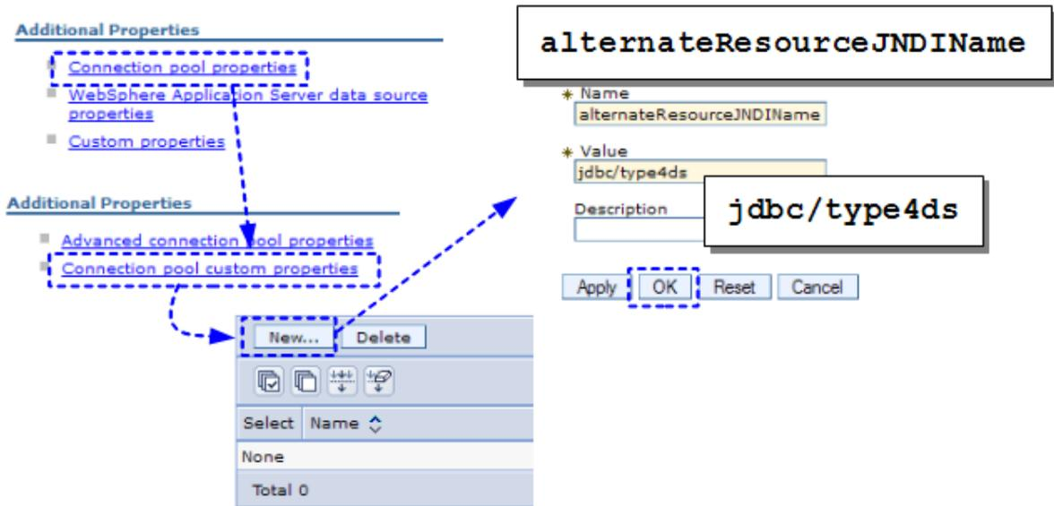
**Note:** A new property in V8. This tells WAS what JDBC data source to use (`jdbc/type4ds`) in the event the primary one (`type2ds` in this case) fails. We are illustrating local Type 2 as the primary with a alternate of a Type 4 connection across TCP.
