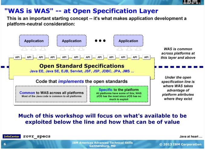
This conveys a very important point about WAS on z/OS compared to WAS on other platforms. Some may think that implies a different programming model, but that's incorrect. The programming model is the same for WAS z/OS as it is for WAS on Windows as it is for WAS on Linux. The exact same Java EE open standards are supported across all the platforms supported by WAS.
