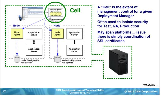
Now we're ready to define what a "cell" is, even though we've mentioned that term several times before. The "cell" is the extent of management control for any given instance of the Admin Console administrative application, which runs in a Deployment Manager. For any given Deployment Manager the master configuration for that Deployment Manager understands what nodes and servers it managed by the XML it sees in the configuration.
