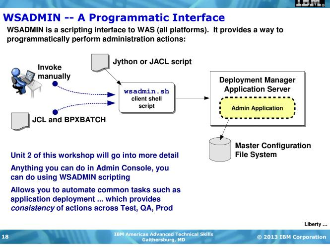
Up to this point we've referred to the Admin Console web application as the means by which configuration changes are made. But there's another method available to you -- the WSADMIN scripting interface. This allows you to use scripts to programmatically perform configuration actions. In Unit 2 of this workshop we'll discuss WSADMIN in a bit more detail.
