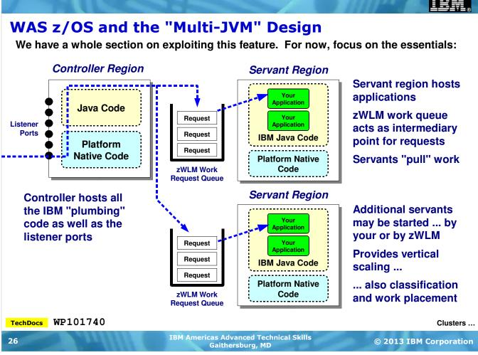
One of the most striking differences between WAS on z/OS vs. WAS on other platforms is the "multi-JVM" model of the application server. On other platforms the "application server" is a single JVM while on z/OS the application server is at least two JVMs and potentially more.
