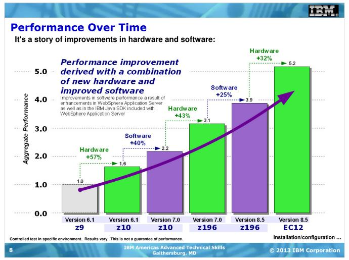
This chart is showing the performance improvements seen in WAS over time with changes in two variables: (1) the version of WAS z/OS and (2) the hardware platform on which the test was run. The trend is obviously upward. The end-to-end improvement is a factor of over five times better performance.
