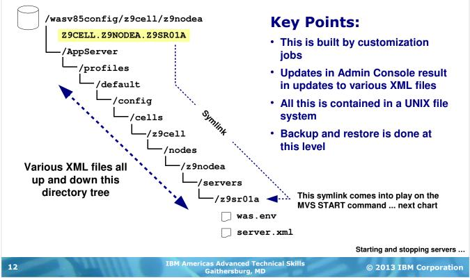
At the heart of a runtime environment is a UNIX file system populated with directories and XML that represent all the customization you provided at time of construction and and any updates you did after the runtime was built. Understanding all the details of this file system is *not* important. At first it's enough to know that the file system consists of a bunch of directories and files, and that the administrative console application understands everything and knows where to put things.
